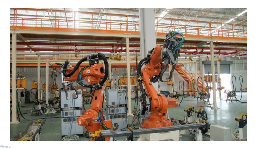
AC 3G-servo robot guns with ABB robot at Aapico Hitech Rayong Plant For Ford T6 Pick Up Truck Project
