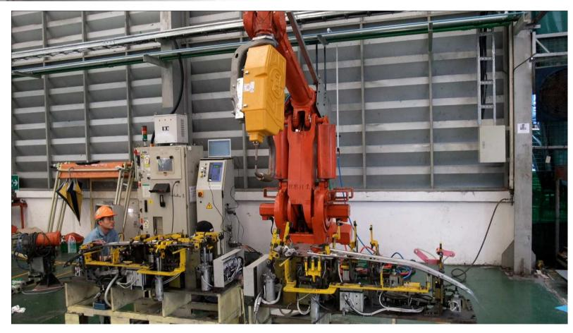
AC 3G-servo 3G gun + iBox controller with 6 AXIS ABB robot at
