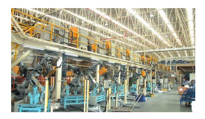
AC 3G servo 3G gun + controller with MOTOMAN robot at Thai Summit Eastern Seaboard for FORD C 346 project
