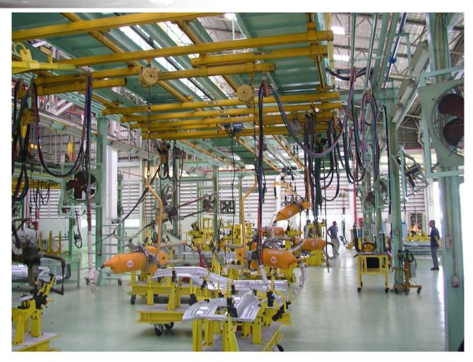
Manual MF Auto adaptive guns and cabinets at Thai-Swedish Assembly Ltd for Volvo Trucks Project
