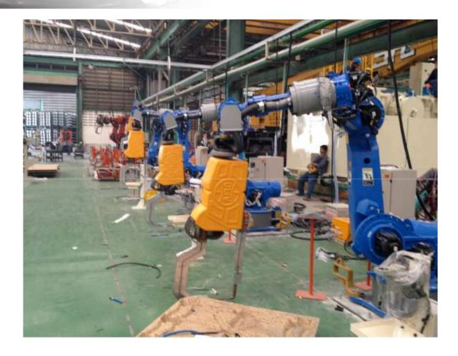
AC 3G-servo 3G gun + controller with MOTOMAN robot at Thai Summit Auto Part industry Bangna Ltd for Nissan Eco-Car Project
