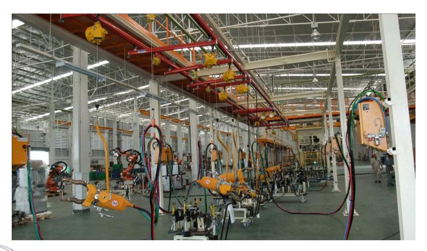
Manual AC guns and cabinets at Aapico Hitech Rayong Plant For Ford T6 Pick Up Truck Project
