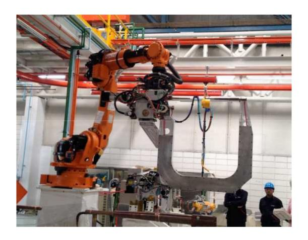
MFDC servo robot gun + MFDC controller with NACHI robot at Thai-Swedish Assembly Ltd for UD Trucks Project
